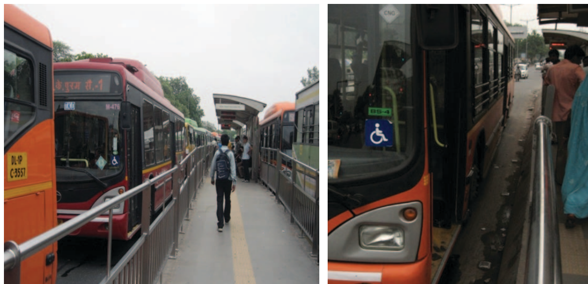
Figure 3.17 (L) Bus pile up at stations (R) Gap at platforms
