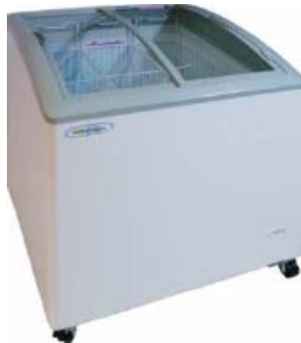
Figure 7. Packaged horizontal ice cream freezer with lids (category IHF6 according to EN ISO 23953), with a net volume of 291 litres, operating in temperature class L1 (-23°C to -18°C), using R507 as refrigerant. Plug-in type.
