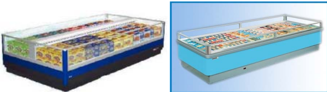
Figure 5. Open remote horizontal frozen island (category RHF4 according to EN ISO 23953), with 7 m 2 TDA (left hand side), operating in temperature class L2 (-18°C to -12°C), using R404a as refrigerant.
