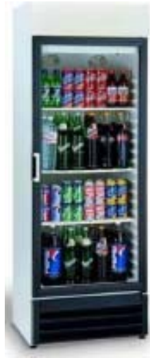
Figure 6. Beverage cooler with one glass door, operating at temperature classes H1 and H2 (5°C), with a net volume of 500 litres, using R134a as refrigerant. Plug-in type.
